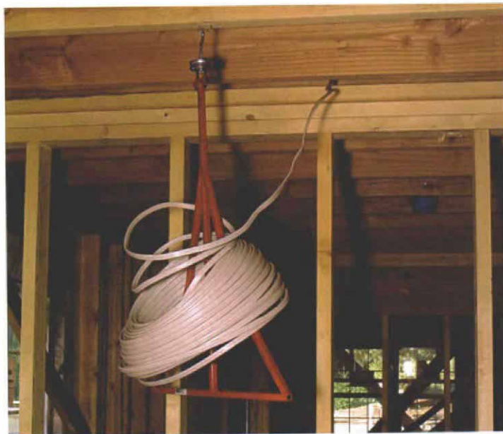
Wire wheel speeds the work. This tool (Mitchell Cryogenics; 816-795-7227; $75) feeds wire from 250-ft. coils without snags or kinks.
